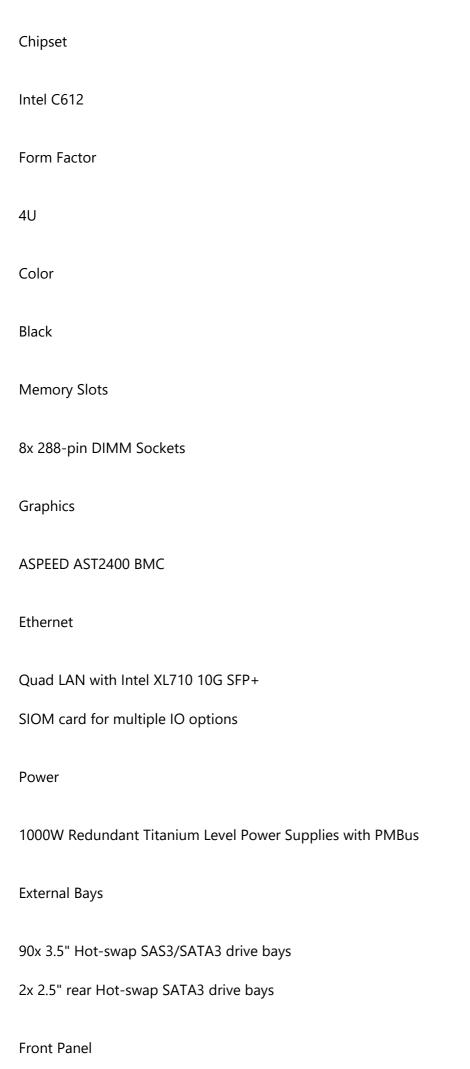
Unit Identification (UID) button Power status LED Hard drive activity LED Network activity LEDs System information LED Power fail LED Back Panel 2x USB 3.0 ports 2x USB 2.0 ports 4x 10G SFP+ LAN ports 1x RJ45 Dedicated IPMI LAN port 1x VGA 1x serial port SAS 12Gbps Controller LSI 3008 SAS 12Gbps Ports 16 SATA 6Gbps AHCI Controller Intel C612 SATA 6Gbps AHCI Ports
